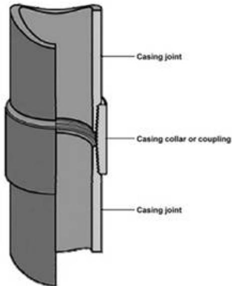
*Connecting Joints of Casing*
